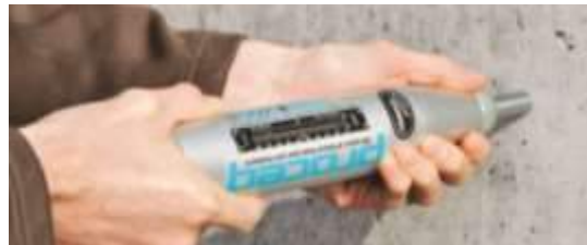
Figure 3. Schmidt hammer test.
